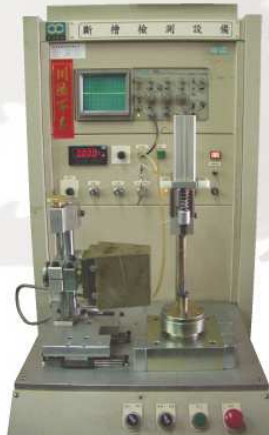
斷槽檢測設備 Rotor Measuring Instrument
