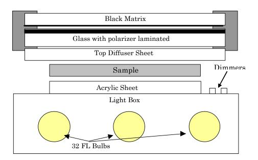
5.2.8.1 Light box: Lumimed LD12AD Viewbox with two banks of 16 EEFL bulbs (Toshiba) apiece. Total viewing surface of light box is 28" X 17" (L X H).
