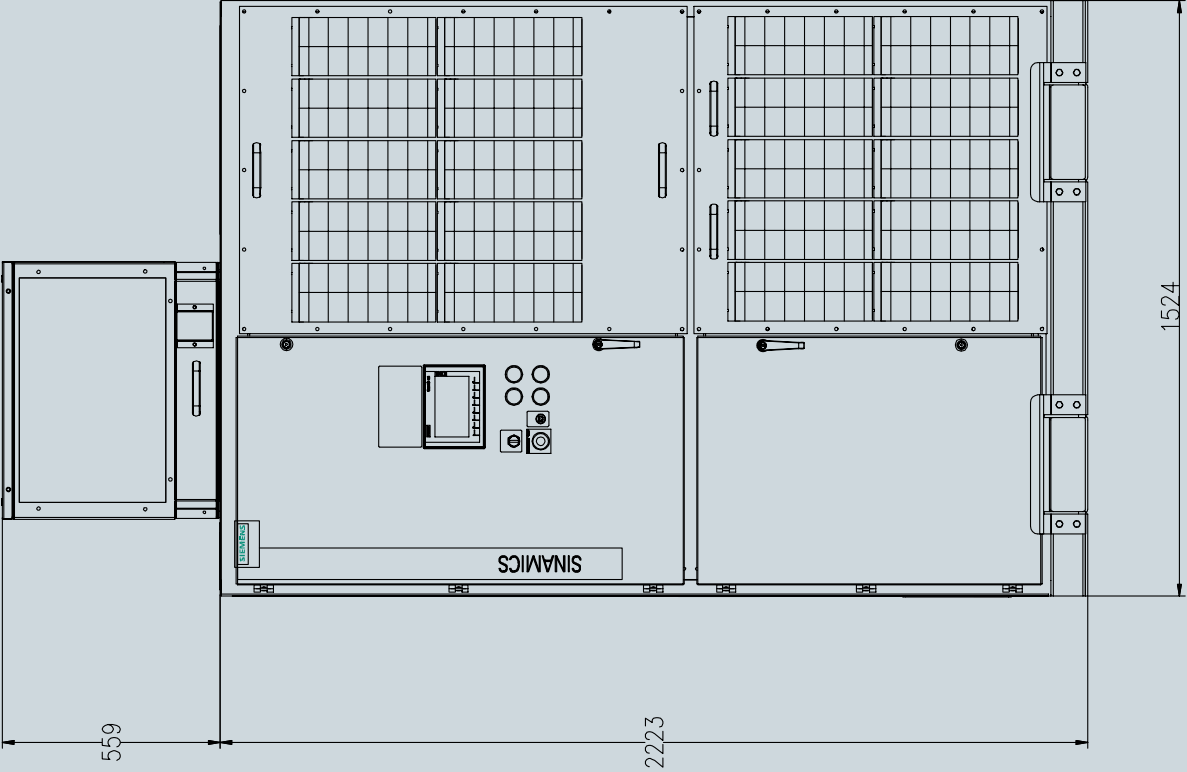
Outline A_ 1524mm x 1067mm x 2782mm (W x D x H)
