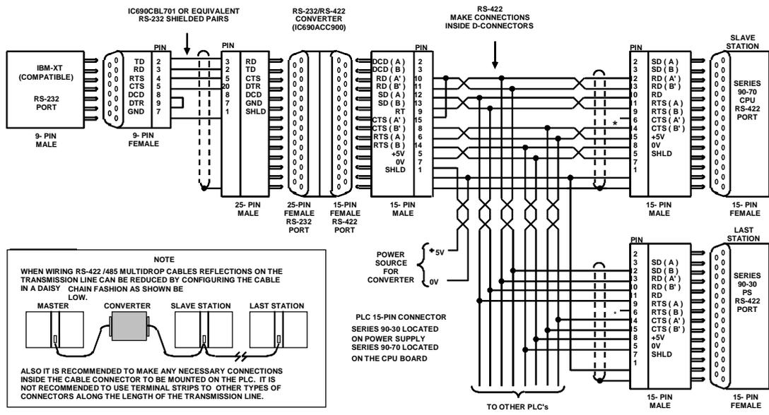
1 TERMINATION RESISTANCE FOR THE RECEIVE DATA (RD) SIGNAL NEEDS TO BE CONNECTED ONLY ON UNITS AT THE END OF THE LINES. THIS TERMINATION IS MADE ON THE SERIES 90 PLC PRODUCTS BY CONNECTING A JUMPER BETWEEN PIN 9 AND PIN 10 INSIDE THE 15-PIN D-SHELL WITH THE FOLLOWING EXCEPTION. FOR SERIES 90-70 PLCs, CATALOG NUMBERS IC697CPU731 AND IC697CPU771, THE TERMINATION FOR RD AT THE PLC IS IMPLEMENTED BY A JUMPER BETWEEN PIN 9 AND PIN 11.
