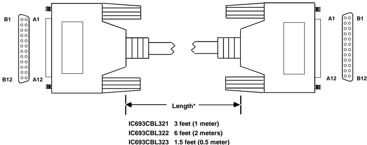
\* Length is measured from backs of connector shells as shown above
