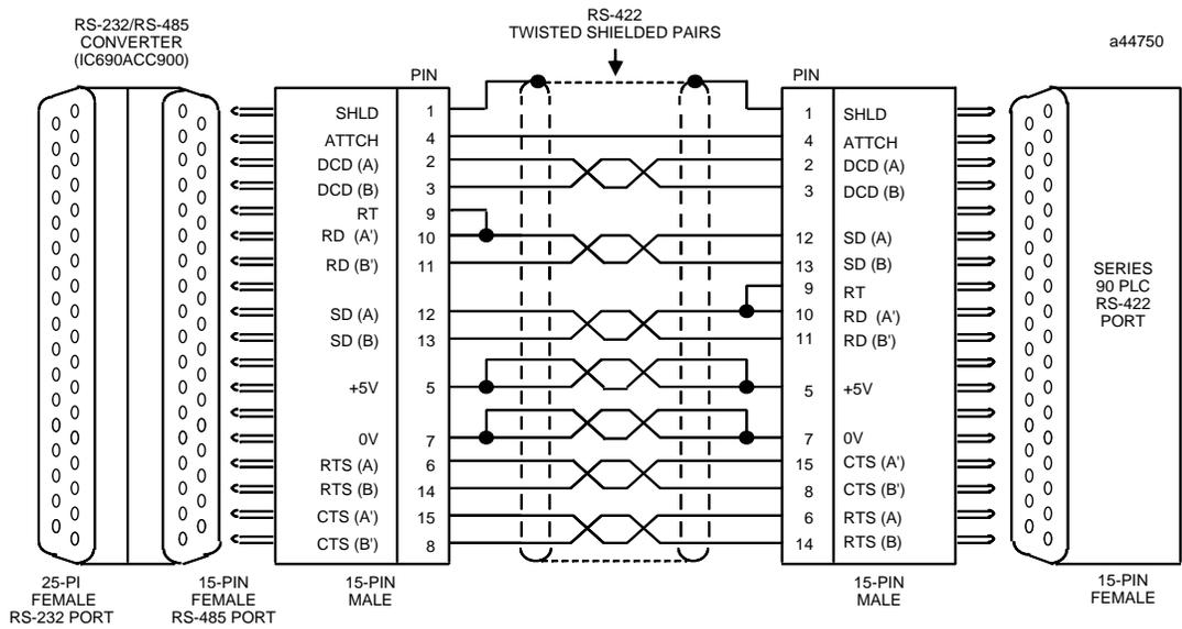
**NOTE:** PINS 9 AND 10 ARE JUMPERED AT BOTH ENDS OF CABLE TO CONNECT TERMINATING RESISTORS FOR THE RD SIGNAL WHICH IS INSIDE THE PLC POWER SUPPLY.
