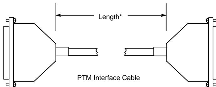
\*Length of IC693CBL340 Cable is 19" (0.50 meter)
