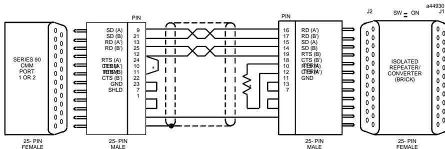
\* TERMINATE CONNECTION: ON THE CMM, INSTALL JUMPER TO CONNECT INTERNAL 120 OHM RESISTOR. ON THE ISOLATED REPEATER/CONVERTER, INSTALL 150 OHM RESISTOR (SUPPLIED).
