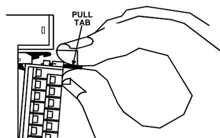
2. Grasp pull-tab towards you until contacts separated from module housing and hook disengaged for full removal.
