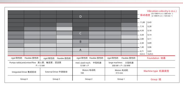
DIN ISO 10816: Mechanical vibrations – assessment of the vibrations of machine through measurements on no rotating parts DIN ISO 10816: 机械振动——通过测量非旋转部分评估机器的振动
