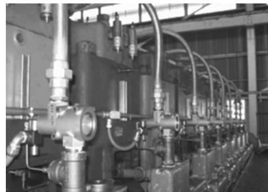
Cam actuated start valves with pressure-actuated in-head check valves
